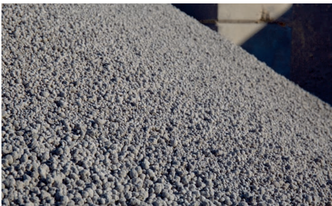
Carbon negative M-LS aggregate from O.C.O Technology is in demand as a sustainable building material
