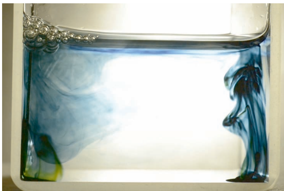
Dyes are used to reveal the concentration levels of carbon dioxide in the water. On the left side is a gas-attracting material, and the dye shows the carbon dioxide stays concentrated next to the catalyst.
